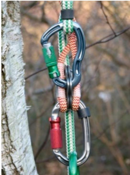
An Oval here has the advantage that it can accept wider loads at both ends, so it can be rotated if desired. And the load from the splice is transferred through the rigging plate of the pulley to a central position on the Oval karabiner where the loading pattern is now  $\frac{1}{4}$ - $\frac{1}{2}$ - $\frac{1}{4}$ , which plays to its strengths. Oval karabiners loaded like this often break at well above their rated MBS
