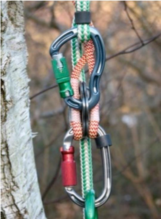
When the climbing line is in tension, both karabiners tend to be pulled into vertical alignment. When ascending, slack may form in the rope
